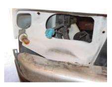
Step 9: Remove the headlight from the car.
