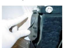
Step 3: Remove the three push pins holding the dust cover from the frame.
