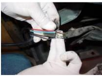
Step 12: Splice (2) power wires to brown wire on parking light connector. Splice (2) black wires to black wire on parking light connector.
