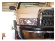
Step 15: Bolt on the headlight and check all functions before driving.
