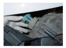
Step 8: Twist off the headlight bulb from the housing.
