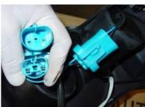
Connect the high beam and low beam plugs, check connectors for proper install.
