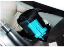
Step 13: Plug the headlight wire harness into the original headlight harness.
