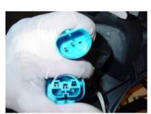
Step 10: Plug the supplied 2 to 1 wire harness into the new head light.
