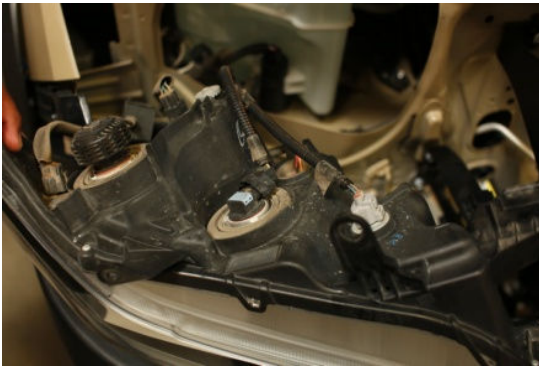
Step 12: Disconnect all wiring connections from headlight and remove headlight (Repeat process on other side)
