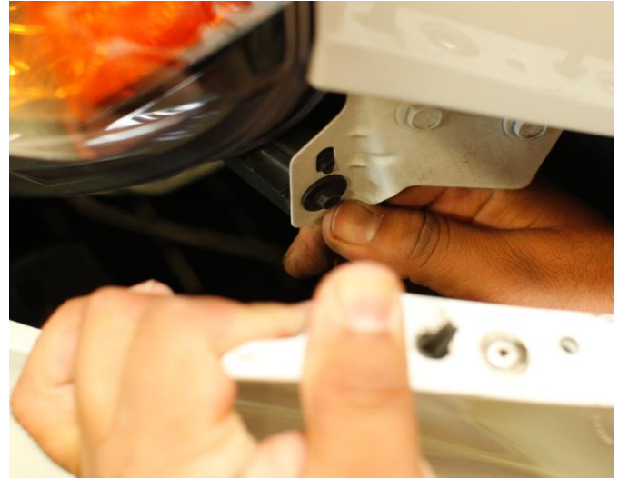
Step 11: Remove second 10mm bolt located between fender and bumper.
