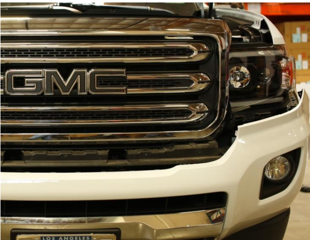
Step 14: Install the Anzo headlight and connect the one OEM harness to headlight and repeat step 12 thru 10 in reverse to secure the Anzo headlight.
