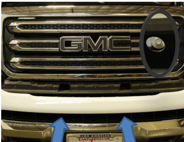
Step 8: Remove two 10mm bolts located within the air dam, near the front license plate.
