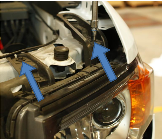
Step 12: Remove two 10mm bolts from on top of headlight.
