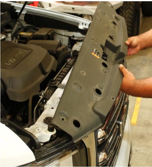
Step 3: With the fan shroud loose, remove fan shroud and place in a safe area.
