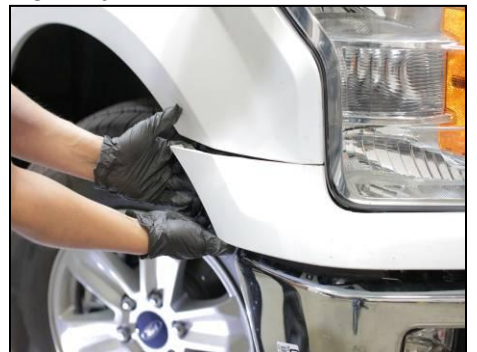
Pull lower valance outwards to unclip from vehicle. Repeat on opposite side.
