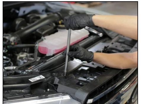
Remove four 10mm bolts on top of radiator grill.
