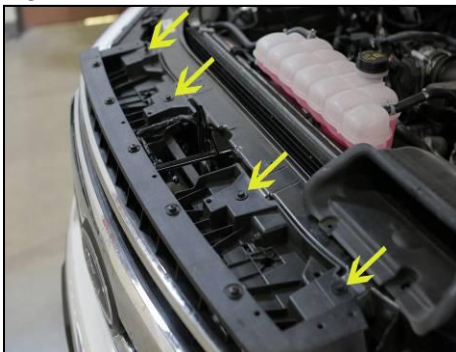
Location of four top 10mm radiator bolts.
