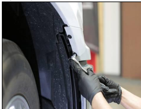
Remove two 7mm bolts in fender well holding lower headlight valance.
