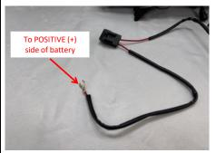
Locate provided Initiation harness (Fig 2) and connect the harness to each side of new headlights as shown. The short side will go to the passenger side and longer side to the driver side as shown in Fig 1.
