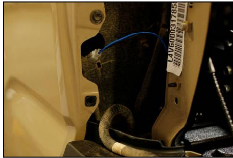
Using mild soap or rubbing alcohol clean surface in fender well then remove tape backing and attach resistor in fender well.
