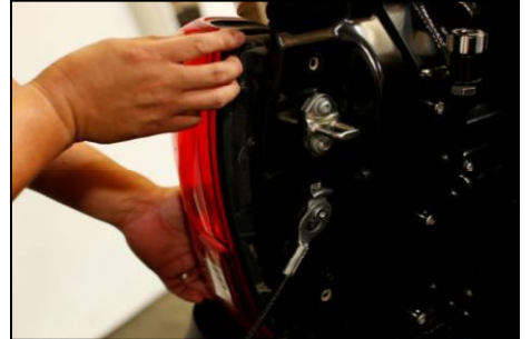
Pull tail lights towards back of vehicle to remove.
